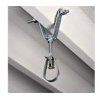
The 115 Standard Duty Loop Hanger is ideal for suspending stationary, non-insulated pipe lines, including CPVC pipes, in fire sprinkler systems. A knurled insert nut helps simplify vertical adjustments and flared edges on the base [1/2" to 4" sizes] help protect pipes from coming into contact with any sharp edges of the hanger.
